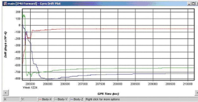
Figure 5.27 IMU Gyro Drift Plot
